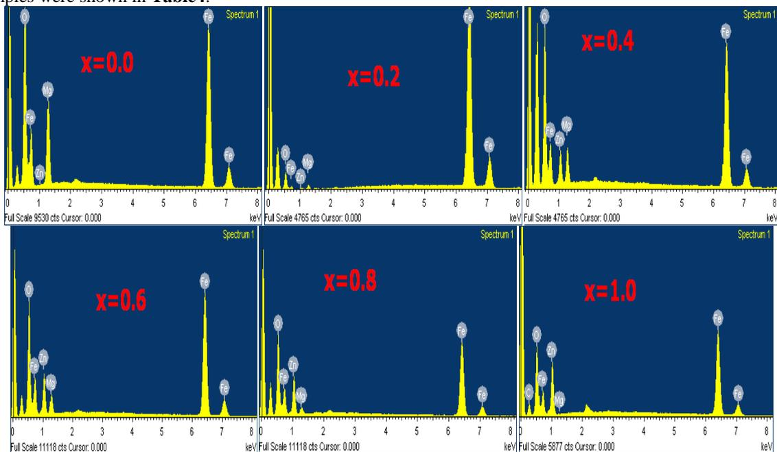
**Figure6. Mg<sub>1-x</sub>Zn<sub>x</sub>Fe<sub>2</sub>O<sub>4</sub> EDS with composition**
